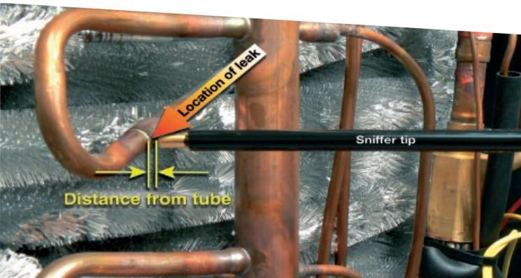
Leak rate signal for leak on backside of a 6 mm (0.25 in) tube joint, leak size  $1 \times 10^{-4}$  mbar l/s (i.e. 22 g/a R134a)
